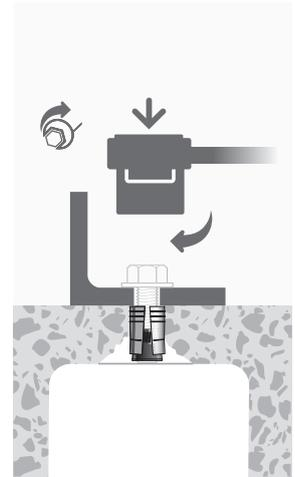
Remove setting tool or bolt and attach fixture using appropriate bolt.
