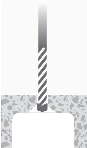
Drill a hole through the concrete into the core using a masonry bit of the correct diameter and tolerance.
