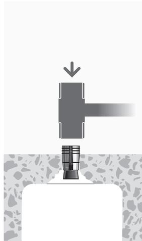
Insert cone end and tap until anchor is flush to the concrete surface.
