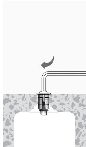
Attach setting tool or bolt and washer onto anchor and expand it by turning the hollow setting tool or bolt 3 to 4 turns or until snug.
